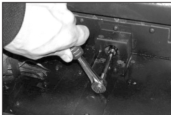
Figure 14: Removing the orifice.
